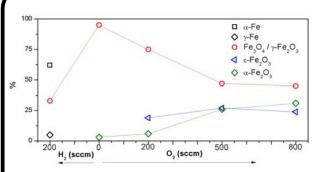
XRD spectra evaluation showing dependence of phase composition on added hydrogen or oxygen into reaction chamber. It's clear that optimal conditions for maghemite synthesis are in pure precursor/argon mixture. XRD cannot distinguish between maghemite or magnetite.
