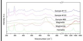
With increasing flow rate production we also increase production of hematite as seen from XRD analysis. We have also used Raman spectroscopy to determine maghemite/magnetite from which is clear that smaple is maghemite based with hematit which was already seen from XRD.
